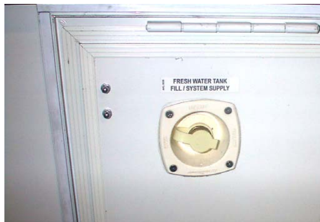
Figure 35: Fresh Water Connection
